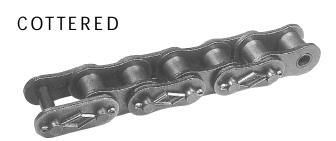
Cottered chain is assembled by staking the pin heads on one side of the chain and drilling a hole in the other end to accommodate a cotter pin. This type of chain is easily assembled and disassembled in the field.
