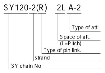
Plain chain consists of "SY chain No" and "Type of pin link". Attachment chain has one space between "Type of pin link" and "Space of attachment".
