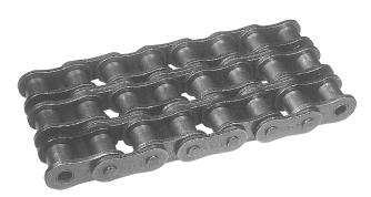
On multiple-strand types, all center plates are slip fitted(clear-ance-fitted) unless otherwise specified.
